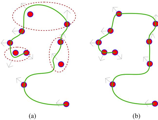
Fig. 4: **Comparison** - Given the same number of points the unified method allows the creation of splines or surfaces that deviate from the constrained (positional) way-points while also representing orientational details to meet the fitness (tuning) criteria. (a) Shows the desired path given the positional points and orientations using the unified dual-quaternion spline. (b) Separate position and orientation spline is unable to match the path without adding additional position way-points.
