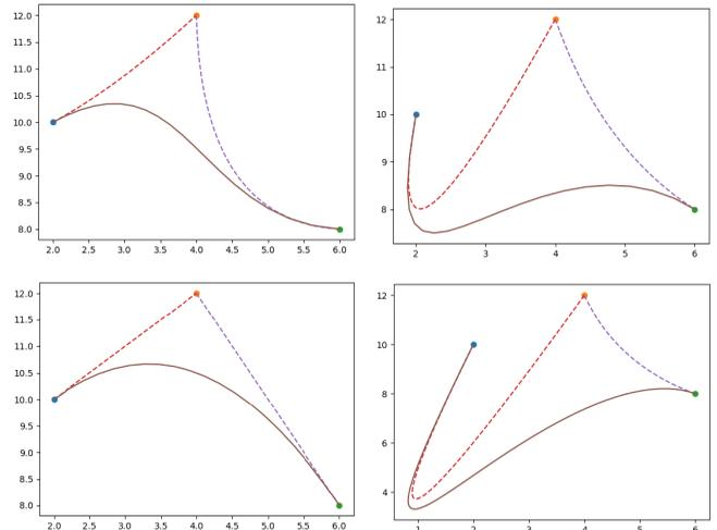
Fig. 3: **Dual-Quaternion Control Points (Curves)** - Three control points with a plot of the intermediate points for the surface. While the example illustrates a quadratic Bézier (i.e., 3 points), a cubic Bézier curve with 4 points (or more) is possible. Dotted line shows the interpolated path between the control points. (bottom-left) orientation for all the control points is the same.
