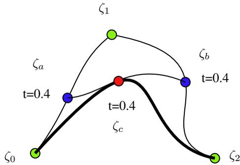
Fig. 2: De-Casteljau's Algorithm for a Curve (using dual-quaternions).
