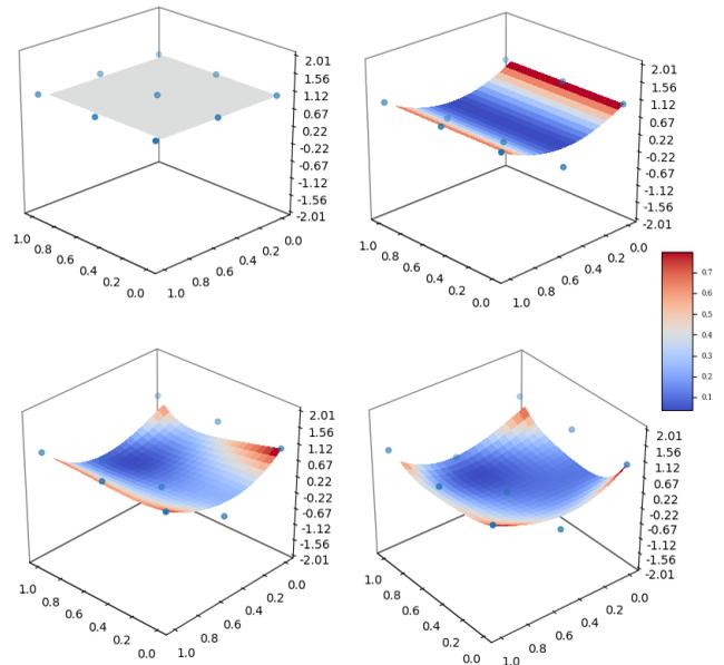
Fig. 5: **Dual-Quaternion Control Points (Surface - 3x3 Control Net)** - (Top left) flat surface with identical orientations), (Top right) control point positions are moved around (orientations kept the same), (Bottom Left & Right) show the control point positions are kept the same while the rotational information is modified.
