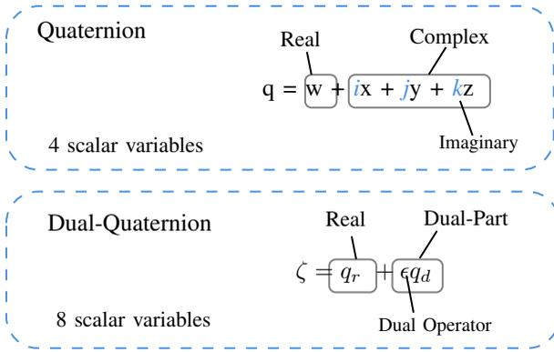
Fig. 1: Visual Overview of Quaternion and Dual-Quaternion Components.
