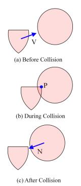
Figure 3. Collision - Resolving interpenetration
