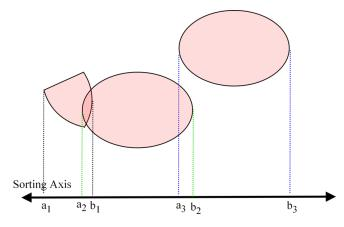
**Figure 2.** Sort and Sweep - Sorting along each of the primary axes.
