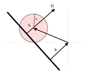
Figure 6. Sphere-Plane - Detecting and gathering contact information for a sphere-plane collision
